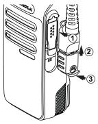
**2** To remove the accessory connector, refer to the steps shown in the diagram.
