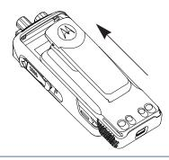
**2** To remove the battery, turn the radio off. Move the battery latch (A) into unlock position and hold, and slide the battery down and off the rails.
