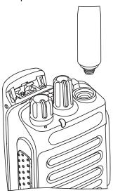
2 To remove the antenna, turn the antenna counterclockwise.
