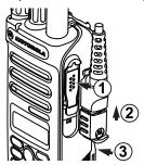
**2** To remove the accessory connector, refer to the steps shown in the diagram.
