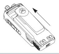
**2** To remove the battery, turn the radio off. Move the battery latch (A) into unlock position and hold, and slide the battery down and off the rails.
